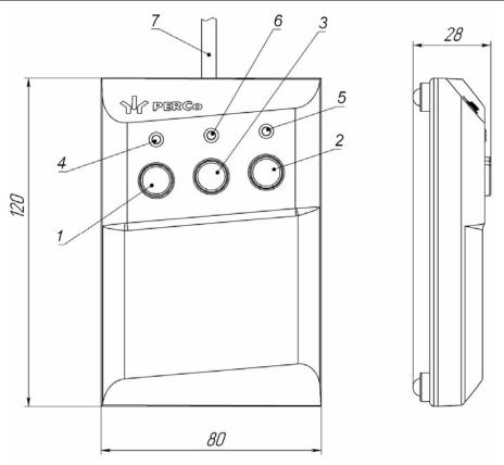
Figure 3. RC panel overall view
