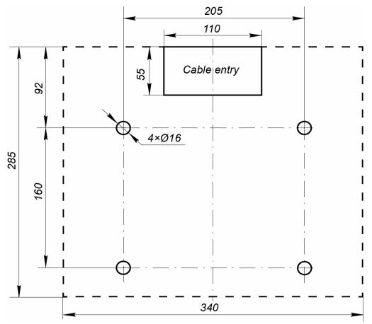
Figure 10. Floor anchor position and cable entries for housing installation (turnstile housing is dotted)
