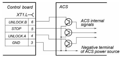
Figure 6. ACS control element — circuit with open-collector output
