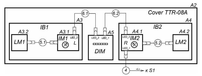
Figure 13. Turnstile cover connection layout
