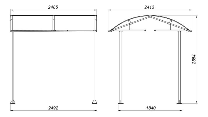
Figure 1. Overall dimensions of the canopy
