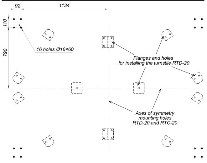
Figure 3. The layout of the holes for the installation of the RTC-20 canopy: 16 holes Ø16×60 – holes for fixing the canopy posts of *RTC-20*
