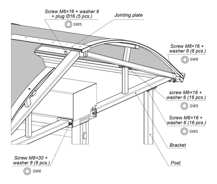
Figure 4. Juncture of the canopy to the turnstile top channel
