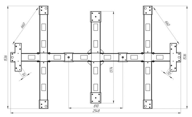
Figure 1. Overall and installation dimensions of the frame
