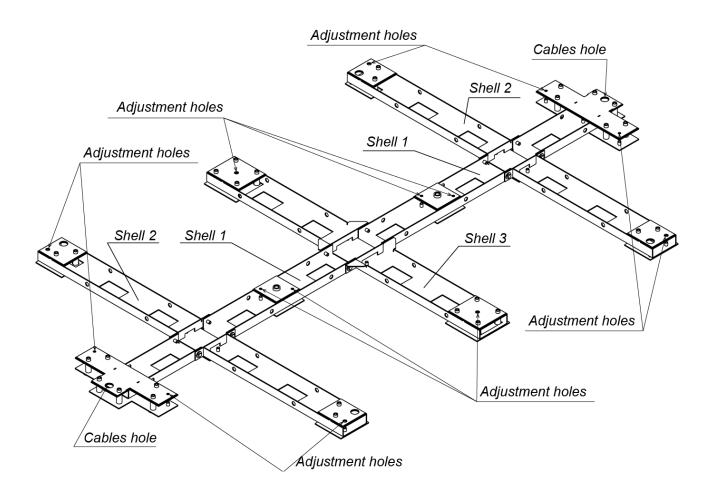
Figure 2. Assembly scheme.
