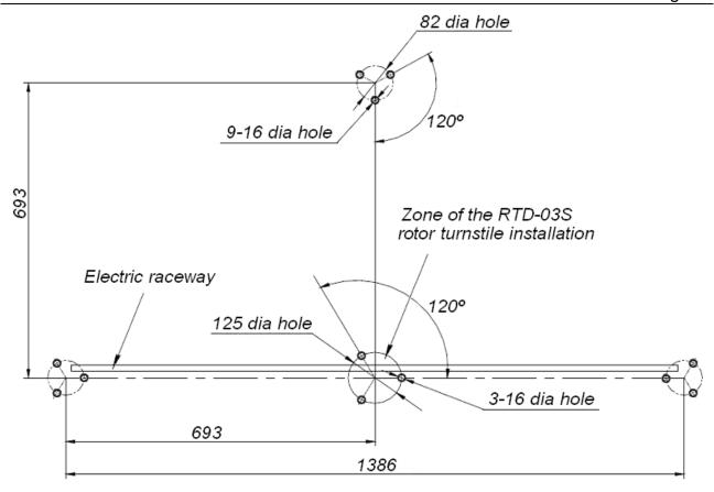
Figure 3 Marking for mounting of the Railing set posts
