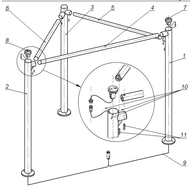
Figure 2. Railing set installation
